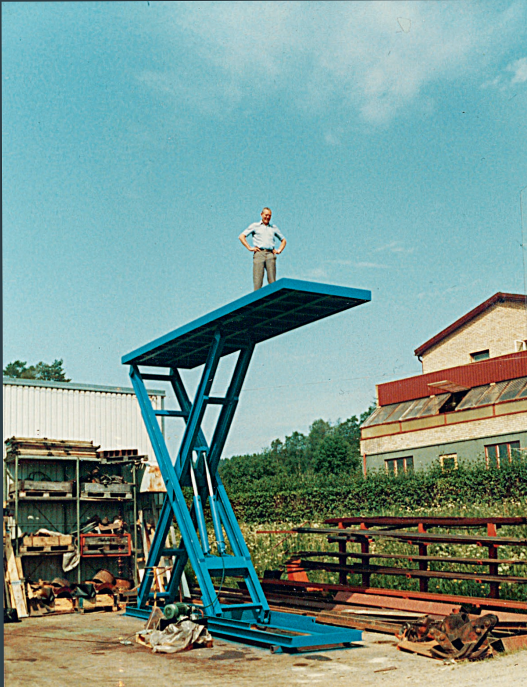
A REALLY HIGH LIFT TABLE FROM THE 1970S. Since then EdmoLift has developed the technique of lifting high even further with vertical double, triple and quattro scissors that can reach as high as 8 metres.
