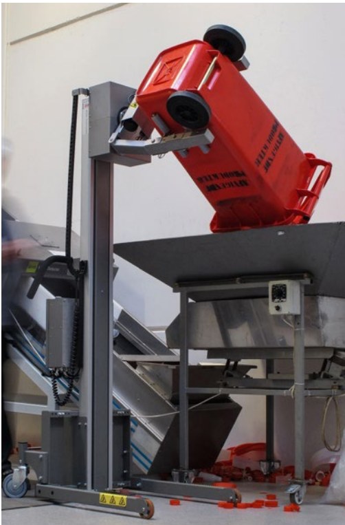
Drum turner 87924 with motorized grip and rotation
