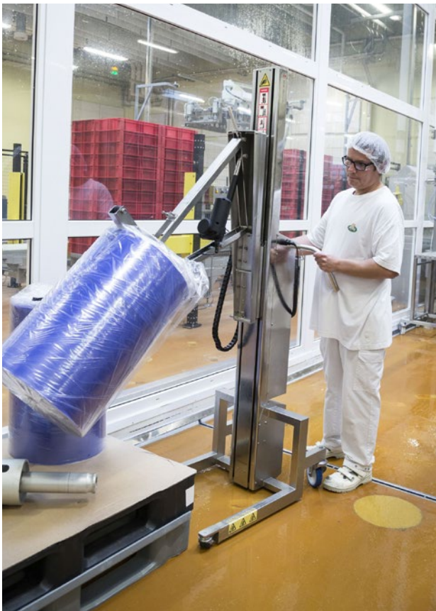
Reel handler 87923 with motorized expansion and rotation
