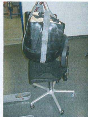
Test Number 8 Functional and proof load
