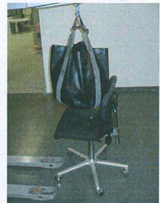
Test Number 8 Functional and proof load
