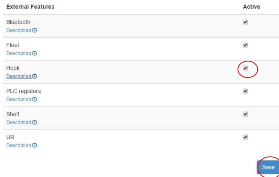
Figure 9 - To be able to set up the robot for transportation of trolleys, make sure the **Hook** feature is activated.
